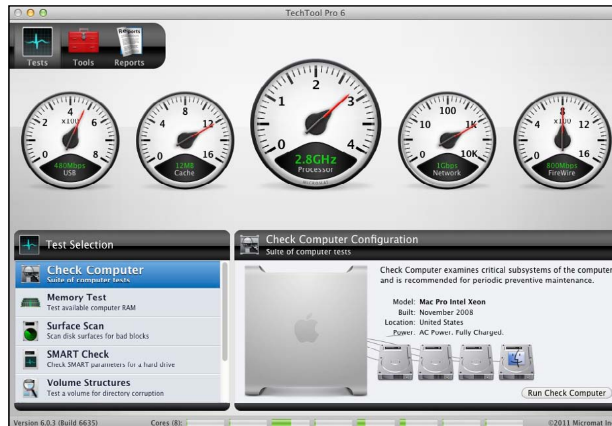
Figure 1. This opening screen is also a diagnostic screen. It indicates that TechTool Pro is running on a Mac Pro with four drives, that the USB ports are running at 480 megabits per second, the CPU has a 12 megabyte cache, the processor is running at 2.8 GHz, the network is operating at gigabit speed, the FireWire port is operating at 800 megabits per second. Along the bottom margin, it indicates that the computer has eight processor cores, only one of which is particularly busy.
